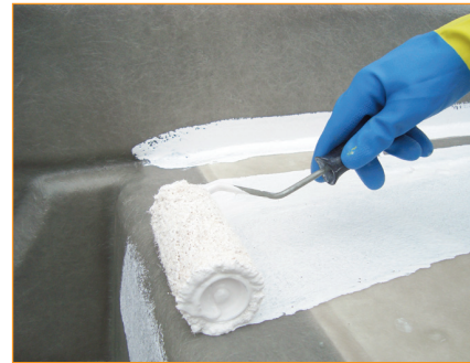
Fig. 3: Laminators at Wright Composites found Crystic® Fireguard 75PA Excel intumescent topcoat easy to apply by brush or with a roller and that it was touch dry "tack free" within 30 minutes
