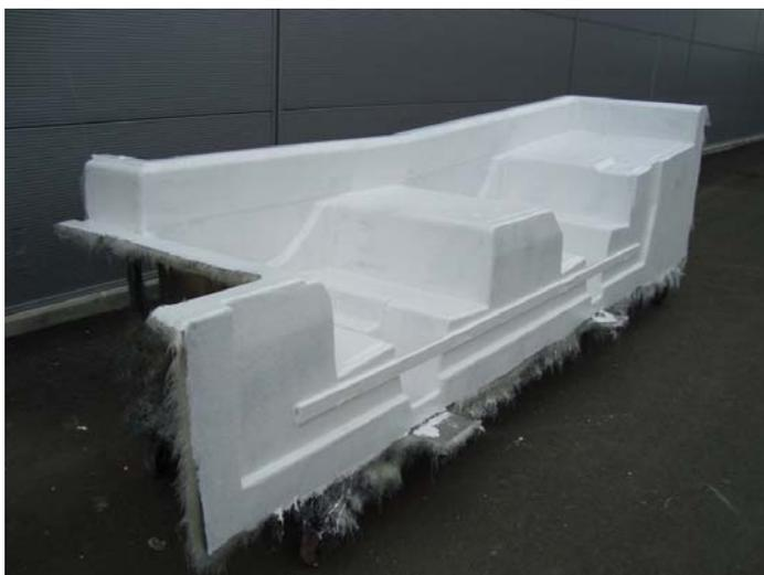
*Wright Composites apply Crystic® Fireguard 75PA Excel FR intumescent topcoat to this rear wheel arch floor section bus part (5 mtr long x 1mtr wide x 1.5 mtr deep. ) to meet the BS474 Class 1 FR specification. [Photo courtesy of Wright Composites.]*
